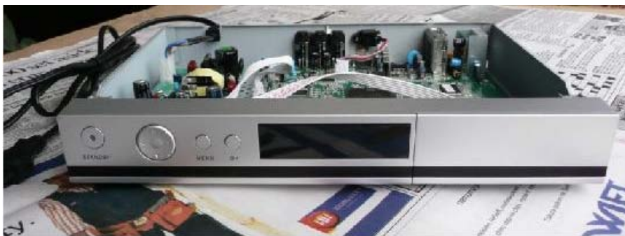
HD DVB-T,DVB-C,DVB-S,DVB-S2 MPEG4 AVC H.264 Set Top Box using ST 7101 Chip with USB2.0
