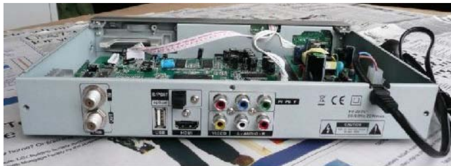
HD DVB-T,DVB-C,DVB-S,DVB-S2 MPEG4 AVC H.264 Set Top Box using ST 7101 Chip with USB2.0
